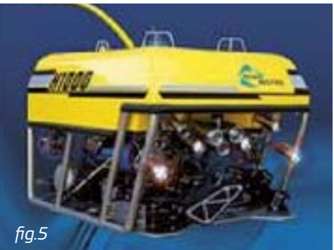
Figure 3: ECA's innovative mine killer with tiltable head Figure 4: ECA OLISTER MIDS Identification and destruction of mines Figure 5: H1000, 1000m rated, remotely controlled subsea inspection vehicle (ROV)
