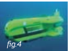
Figure 3: ECA's innovative mine killer with tiltable head Figure 4: ECA OLISTER MIDS Identification and destruction of mines Figure 5: H1000, 1000m rated, remotely controlled subsea inspection vehicle (ROV)
